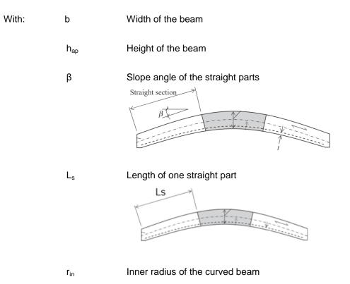
Combined tension perpendicular to the grain and shear in the Apex zone
