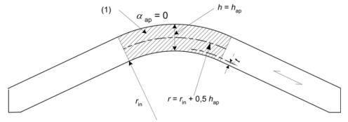
For the sections located at the Apex (all sections in the hatched zone) additional checks are executed:
