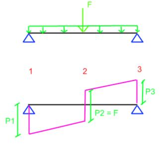
When evaluating the jumps in the shear force diagram of a given member, also the shear diagrams of the adjacent members are accounted for. Adjacent members are defined as neighbouring members within the same buckling system.
