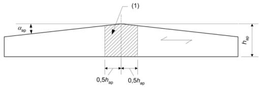
For the sections located at the Apex (all sections in the hatched zone) additional checks are executed:
